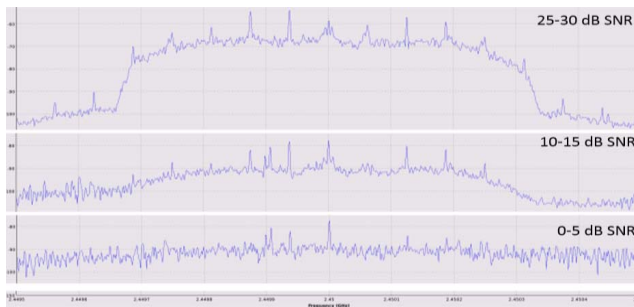
Fig. 2. Example of a modulated signal with three different power levels
