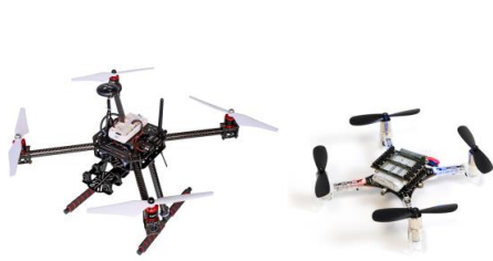
Fig. 2: NXP (left) and Crazyflie (right) UAS platforms used for demonstrating the proposed autonomy framework.
