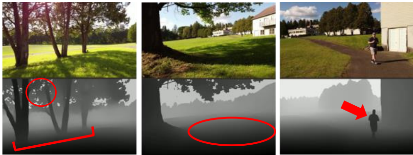
Fig. 3: Examples of disparity estimation (bottom) from RGB (top) and qualitative evaluation features.
