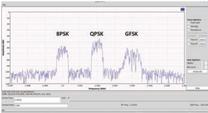
Fig. 8: Spectrum of three simultaneous transmissions
